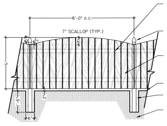
2" X 4" P.T.S.Y. PINE STRINGERS (BEYOND) (TYP.). ATTACH TO POST W/ 2- I6D GALV. SINKERS/ END OF STRINGER (BUTT JOINT STRINGERS @ POST)
